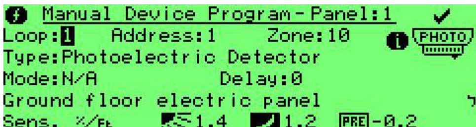
Screen 63 System configuration – manual device program
