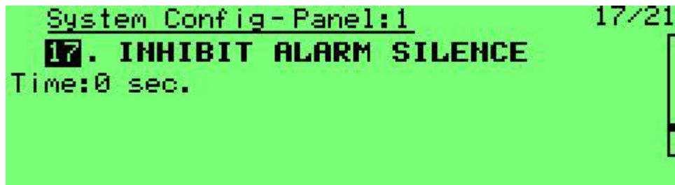
Screen 58 System configuration – inhibit alarm silence
