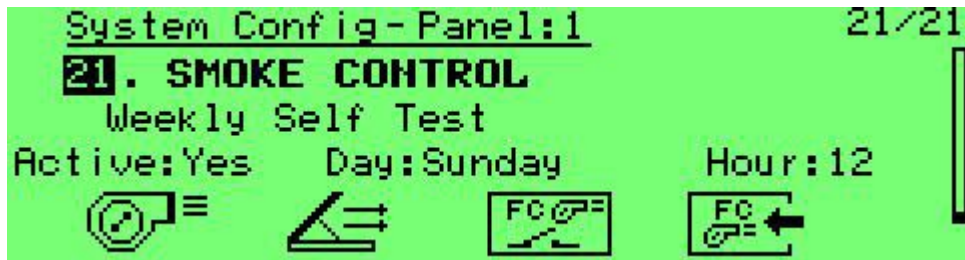
Screen 61 System configuration – Smoke control test settings
