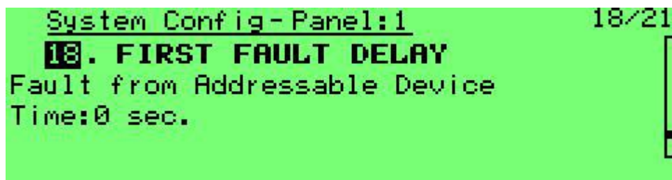
Screen 59 System configuration – first fault delay
